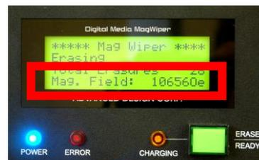
The LCD displays the "Erasure Complete" message showing total number of erasures and magnetic field intensity in: Oe(Oersted).
